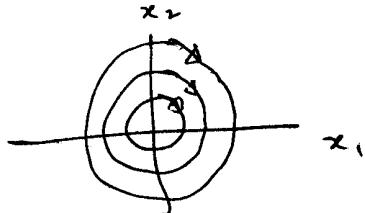
Amplitude of oscillation depends on  $y_0$  and  $\dot{y}_0$
